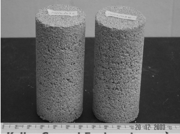
FIGURE 2. The artificial specimens after fired at 500°C for 5 hours in furnace with void ratio of 0.6
